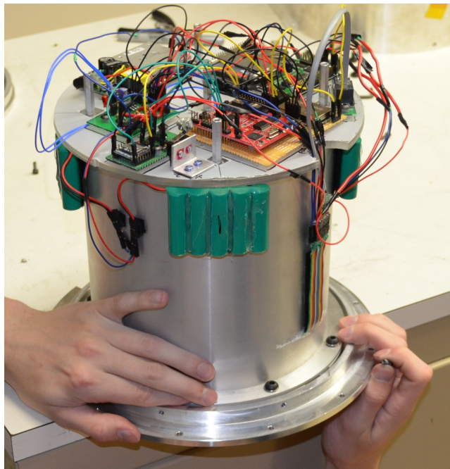
Figure 6: Fully assembled payload canister before wire assemblies are staked down for launch and RockSat canister is attached.
