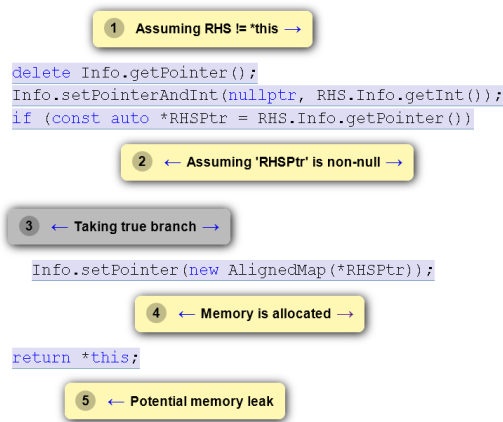
Fig. 4. Emerging error reporting systems like LLVM scan-build provide stark contrast to those of conventional IDEs. Here, scan-build presents error messages for a potential memory leak as a sequence of steps alongside the source code to which the error applies.
